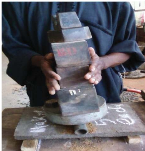
Plate 2.0: Makuba clay roof tile under progressive loading for flexural strength test
