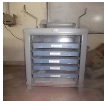
Figure 3. Shaker for Sieving of Aggregate
