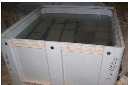
Figure 6. Curing of Concrete Cubes
