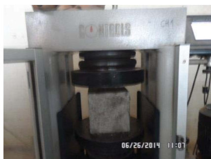
Figure 7. Compressive Strength Testing Machine
